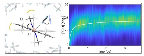
QM/MM BOMD simulations of a prototype Cu(I) bis-phenanthroline complex reveal the coupling between the excited-state flattening dynamics, which controls the efficiency of photosensitization, and the intercalation of acetonitrile molecules between the ligands [5].
